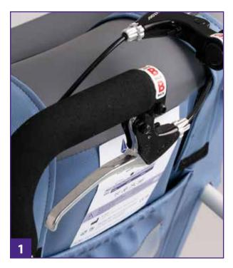
Pull in the 'B' labelled **Backrest Adjustment Lever** and adjust the back as required. Release to set in position.
